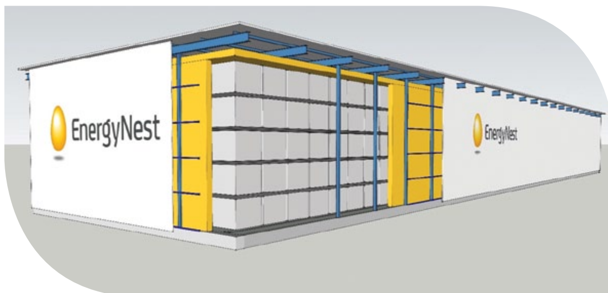
Figure 1: Illustration of a 730 MWh thermal energy storage. Approximate measures are 105 x 25 x 12 meter.
