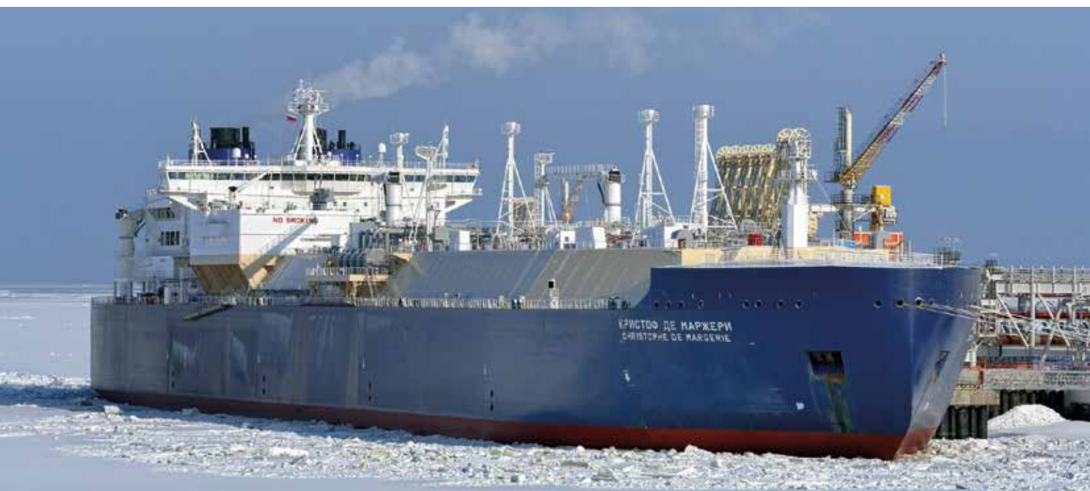
The Christophe de Margerie is capable of sailing through ice up to 2.1 metres thick (Pic: Sovcomflot)
